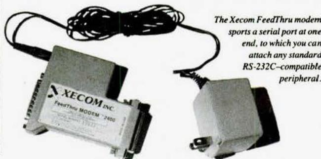
The Xecom FeedThru modem sports a serial port at one end, to which you can attach any standard RS-232C-compatible peripheral.
